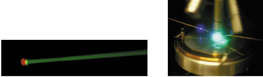
Figure 1.4: Left: first light from Silicon. Nanocrystalline Silicon emits red light when stimulated by an argon-ion laser (green light). Right: experimental setup to observe emission of visible light from Silicon Nanocrystals.
