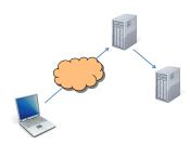
Connection to a remote machine protected by a firewall.  $\operatorname{ssh}$  -t theory  $\operatorname{ssh}$  nero
