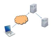
Connection to a remote machine protected by a firewall.  $\mathtt{ssh}$  -t theory  $\mathtt{ssh}$  nero
