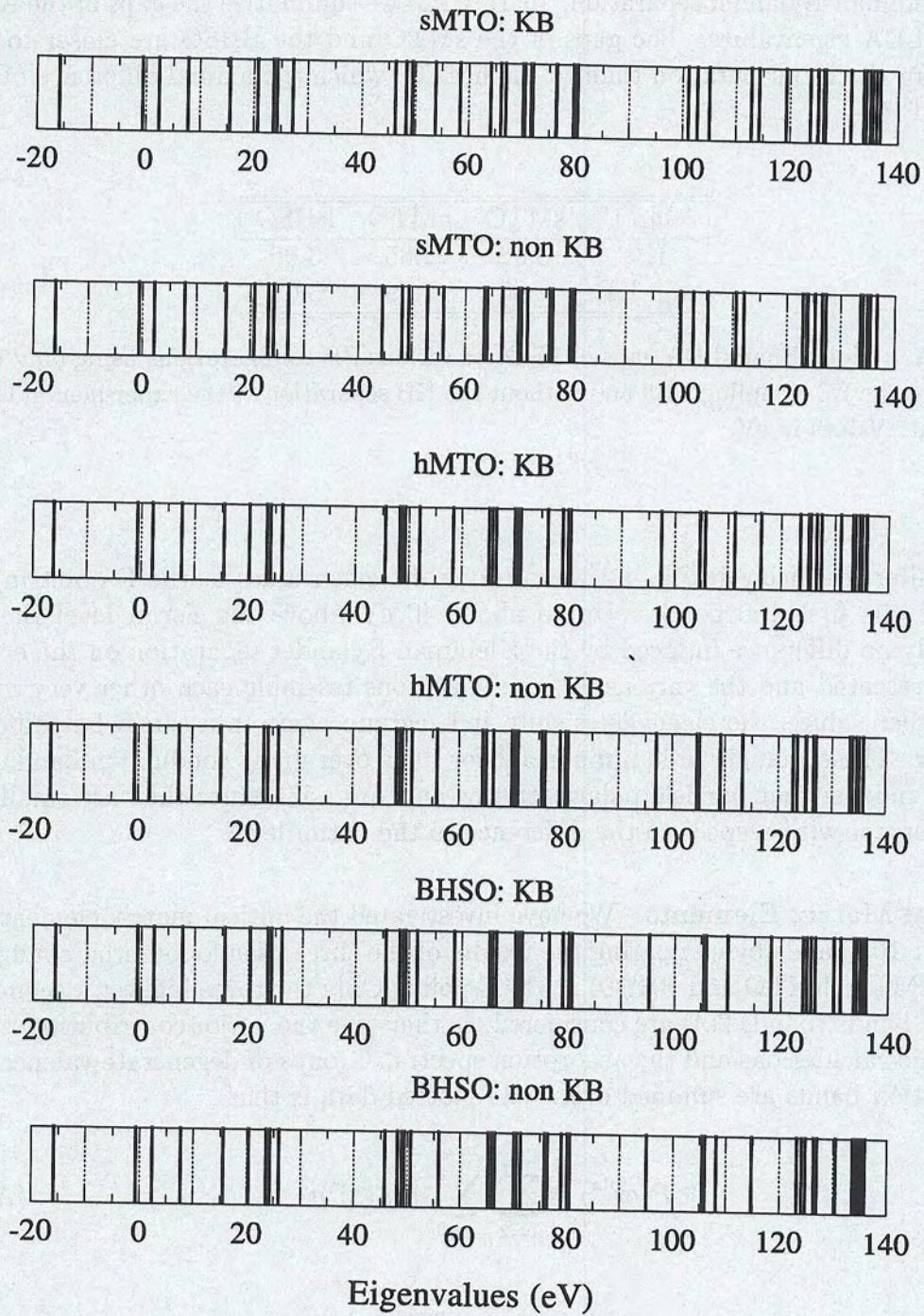
Figure A.4: Comparison of Kohn-Sham LDA eigenvalues of \text{Li}_2\text{O} for the first 100 bands using only the \Gamma point in the BZ sampling with and without the KB separation for various PP configurations at the experimental lattice constant.
